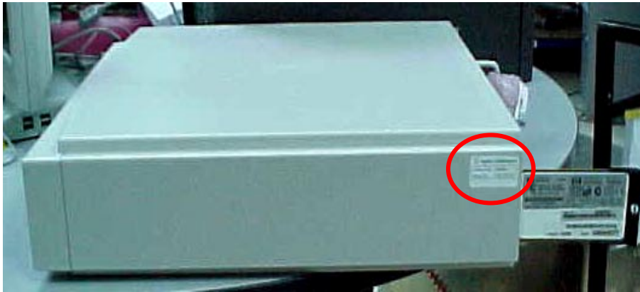
Picture 1. Agilent Serial Number Label Location on B180L UNIX Controller (label is circled)
